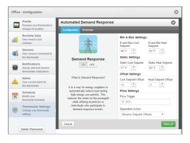
The right column of the ADR configuration page is where the occupant adjusts the operational parameters for ADR. The utility may send up to 3 types of ADR signals to Skyport. These are: 1) Pricing for the cost of energy, 2) An Offset to the occupants' comfort setpoints, and 3) a signal to enforce discrete or Static setpoints.
