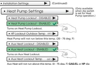
switch must be set for HP and GAS or ELEC dip switch must be set for ELEC.
