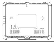
To remove the thermostat backplate: Using the Finger Pull Areas, pull the front housing away from the backplate.
